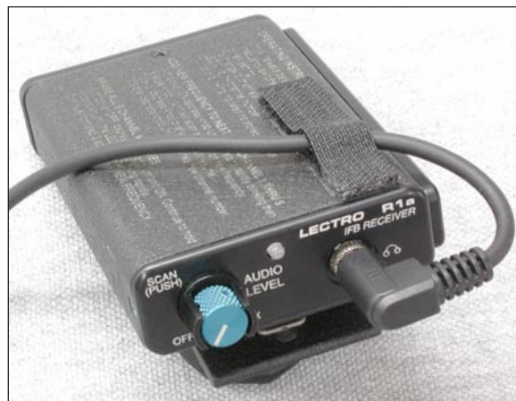
Figure 2 - Headphone cord strain relief
